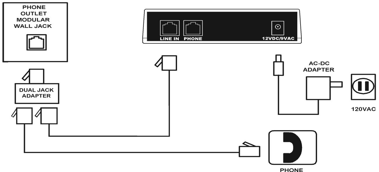
Fig. 2 Connection Diagram for Normal Use
